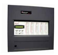
The PARK2000 carbon monoxide detection panels is specially designed for application in garages with 3 up to 5 CO detection zones. Each zone supports a maximum of 16 NC0100 detectors distributed over a line of up to 500m in length, with 1.5mm² cable section, twisted and shielded. They have a control module with an LCD screen that displays the alarm and fault levels of each zone and allows the reading of CO concentration per zone in sequential mode.
