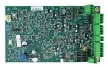
The System IO card provides a VdS DXc panel compliance interface to communicate with the required Fire Brigade equipment as part of the VdS compliant Fire System.
