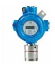
Methane / Ammonia detectors with Infrared sensor and LCD dislpay in EEx certified container. D. Proportional output 4-20mA. Measuring range 0 to 100% LEL. Zero Tracker to counter possible drifts.
