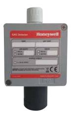
The detector is equipped with a head with a catalytic sensor element that measures the concentration of the explosive gas on the LEL (Lower Explosive Limit) scale.
