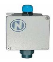
Butane detector in dust-proof box. The catalytic sensor assures alarm signal through 4-20mA proportional output. Can be connected to addressable control panel through suitable module.
