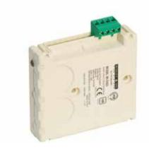
MI/DISO is intended to be spaced between groups of devices on a communication line to protect the line if a short circuit fault occurs. It automatically opens when the voltage in the communication line falls below a fixed threshold. If a short circuit fault occurs, the two isolattors located around the device group where the fault occured will sense the line voltage drop, open their switches and remove the devices from the rest of the line.
