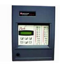
The PARK2000 carbon monoxide detection panels is specially designed for application in garages with 1 up to 2 CO detection zones. Each zone supports a maximum of 16 NC0100 detectors distributed over a line of up to 500m in length, with 1.5mm² cable section, twisted and shielded. They have a control module with an LCD screen that displays the alarm and fault levels of each zone and allows the reading of CO concentration per zone in sequential mode.
