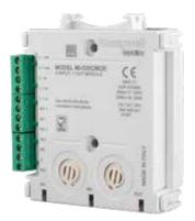
The MI-D2ICMOE provide supervision of one input circuits respectively from external devices; it also provides an unmonitored single pole volt-free changeover contact for external devices. All modules feature a built-in short circuit isolator.
