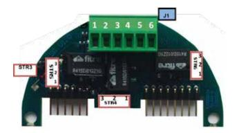
The 3-relay interface gives the possibility to have a dry contact for each single event: alarm, pre-alarm and fault.
