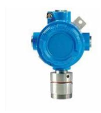
Chlorine / GAS / Butane Gas Detectors with Infrared Sensor. In EEx certified container, suitable for installations in classified AD-PE range 4-20mA proportional output. Measuring range 0 to 100% LEL.
