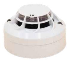
The MI-RHSE-S2I uses the same thermistor and microprocessor technology to provide an alarm when the rate of rise in temperature exceeds  $10^{\circ}$ C/ minute (typical) or if the temperature exceeds a threshold of  $58^{\circ}$ C (Response Class A1R).
