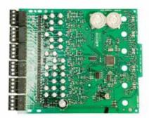
The design of the System Sensor 500 Series multiple input and output modules allows for installation ease and time savings The monitor and control modules can be used to supervise and activate sounders, strobes, door closers, pull stations, waterflow switches, conventional smoke detectors and more. The conventional zone interface module is ideal for retrofit applications to monitor zones of conventional two-wire detectors.
