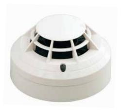
The detector uses the thermister and microprocessor technology to provide an alarm when the rate of rise in temperature exceeds  $10^{\circ}$ C/minute (typical) or if the temperature exceeds a threshold of  $58^{\circ}$ C response Class A1R).
