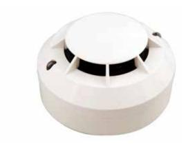
The photoelectric smoke sensor delivers high responsiveness, reduced sensitivity to dust and false alarms resulting from ingress of insect and other debris. The plug-in unit uses sophisticated processing circuitry that incorporates smoothing filters to help eliminate transient environmental noise conditions that can be the cause of unwanted alarms. The devices are managed by embedded software running complex algorithms that further improve resilience to false alarms and improve detection speed.
