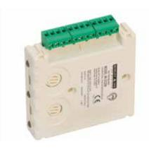
MI/DCZRM addressable zone monitor module allows a zone of non-addressable devices to communicate with Honeywell Morley-IAS protocol analogue addressable system. As a result existing non-addressable zones can be integrated into a Honeywell Morley-IAS protocol system. The module monitors a zone of two-wire non-addresable devices.
