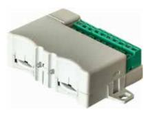
MMT is a 4÷20mA analogue input module for gas detectors and other device interfacement that use this standards. The module is compatible with new NOTIFIER panels series. Each MMT module use only one address of 99 available on loop. Microprocessored Module compatible with Notifier protocol, MMT is designed to manage a single detector. The address codification is achieved through decimal rotative switches.
