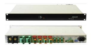
The Emegency Power Supply acts as a battery charger and control device for 24V DC external back up batteries in accordance with EN 54-4+A1+A2 standards. The front panel includes LED indicators, control push button and USB socket, allowing control and test of power supply operating parameters.
