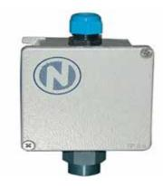
Nitrogen monoxide detector in dust-proof box. The electrochemical cell assures alarm signal through 4-20mA proportional output. Measure area 0 to 30%. Can be connected to addressable control panel through suitable module. Can be used with relay board on double threshold control panel with pre-alarm 10mA and alarm 20mA.
