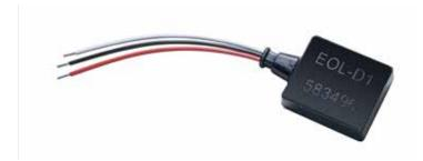
End-of-line module for the end of the VARIODYN D1 voice alarm system loudspeaker line for standard-compliant monitoring, when more than 20 loudspeakers are connected to a line.
