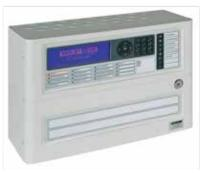
DXc1 is a single-loop fire control panel. It can operate as stand-alone or networked system with other DXc series panels up to 16 loops. Text can be quickly inserted from the panel's mobile phone style keypad to identify the exact location of each field device.
