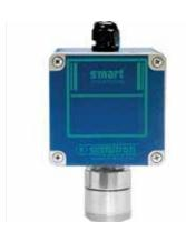
Carbon dioxide detector in dust-proof box. The IR sensor assures alarm signal through 4-20mA proportional output. Measuring range from 0 to 2%. Can be used with relay board on double threshold control panel with pre-alarm 10mA and alarm 20mA.
