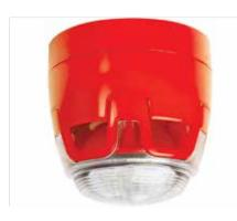
Combined acoustic and optical alarm signaling device, with IP65 Ingress rate protection enclosure is EN 54-3 & EN 54-23 compliant, in red housing, and offers a selection of 32 signal tones including the DIN tone and other country-specific tones. All tones comply with EN 54-3. Tone configuration takes place via a 6-pin DIP switch. Up to two different signal tones may be activated.
