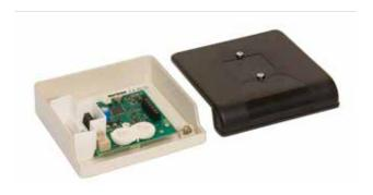
The MI/D240CMO addressable output module provides a single double pole contact output for 240 VAC (nominal 220 VAC) to switches the power to external equipment.
