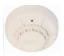
The conventional ECO1004T 78°C fixed temperature thermal detector use state of the art thermal elements combined with application specific integrated circuits (ASIC) to provide quick and accurate detector of fires through temperate levels or changes.
