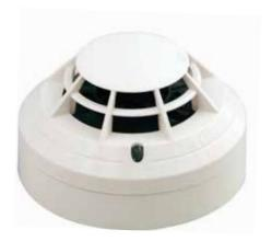
The detector uses fixed temperature analog addressable sensors employing low mass thermistors and microprocessor technology for fast response and linear temperature sensing.
