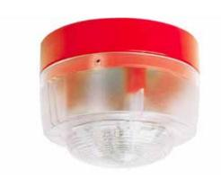
Optical signaling device compliant with EN 54-23 for wall and ceiling mounting with white strobe color and flat base. The signaling device is suitable for square signal ranges W-2.4-9.0 and cylindrical signal ranges C-3-9.5 / C-6-9.5 / C-9-9.5.
