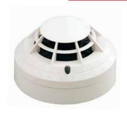
The optical-thermal sensor uses thermal assistance to the core photoelectric smoke detector to give enhanced false alarm immunity and faster response to a wide range of incipient fires. The plug-in unit combines two separate sensing elements that are managed by embedded software to act as a single unit. The optical-thermal detector conforms to EN54-7, a 58°C fixed temperature and rate of rise thermal assistance conforming to EN54-5.
