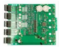
The CZ-6 provides an interface between the intelligent system and a two-wire conventional detector zone. A common SLC device is shared between all modules and the initiating devices share a common external supply; otherwise, each module operates independently. The first address is set from 01 to 94; the other modules are automatically assigned the next five addresses; up to two unused addresses can be disabled.
