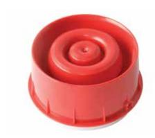
Honeywell Morley-IAS wall mounted sounder is installed in exactly the same manner as an intelligent fire detector. Common installation base (Part No. MI/B501AP/IV), which accepts any product within Honeywell Morley-IAS audiable-visual product family, is installed at first fix. This common base is fitted with a shorting spring, enabling loop continuity to be maintained without having to install any Honeywell Morley-IAS audiable-visual product.
