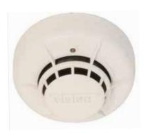
The conventional ECO1003A photoelectric smoke detector uses a state-of-the art optical chamber operating on the light scattering principle, combined with an application specific integrated circuit to provide quick and accurate fire detection.
