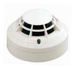
The detector uses the thermister and microprocessor technology to provide an alarm when the rate of rise in temperature exceeds 10°C/minute (typical) or if the temperature exceeds a threshold of 58°C response Class A1R).
