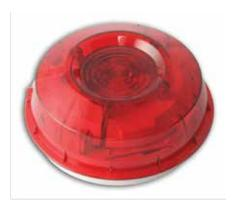
The wall mounted strobe is installed in exactly the same manner as an intelligent fire detector. A separate, common installation base (Part No. MI/B50IAP/IV) which accepts any product within Honeywell Morley-IAS audiable-visual product family, is installed at first fix. This common base is fitted with a shorting spring, enabling loop continuity to be mainteined without having to install any audiable-visual product.
