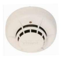
The conventional ECO1002 is a multi-criteria detector uses a state-of-the-art optical chamber and a thermal element combined with a microprocessor, running sophisticated algorithms to provide quick and accurate detection of fires.
